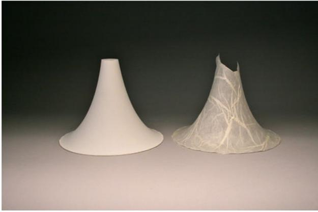
**Figure 3.** Left: the plastic pseudosphere. Right: a sheet of pseudospherical paper after forming and drying.
