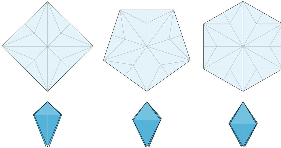
**Figure 5.** Top: Crease patterns for  $N = 4, 5, 6$ -gons. Bottom: The folded origami bases. Note that the flaps (shaded) become shorter and wider as  $N$  increases.
